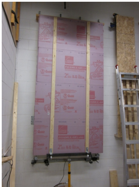
Figure 4. Short-term deflection test panel
